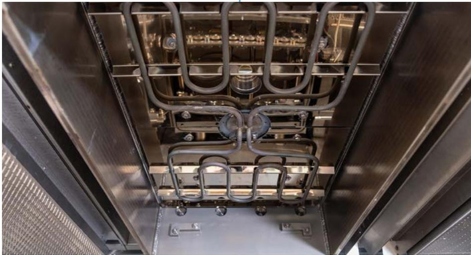
The medium-wave radiant heating system in the vacuum module ensures thermal stability and offers maximum flexibility in profile design.
