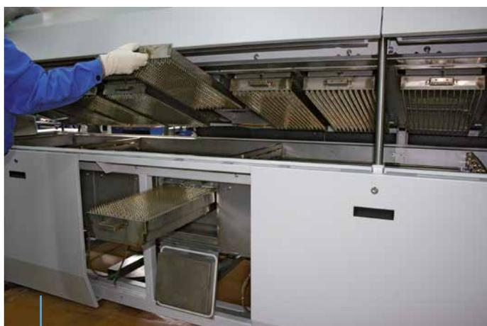
Ersa HOTFLOW 3/14: Optimum access possibilities for fast and straight forward maintenance.
