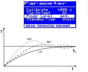
This function enables the user to influence the regulating behavior of the station, whereby the heating and after heating behavior of the station can be matched to the actual application. Three settings are possible: [high], [med.] and [low].
