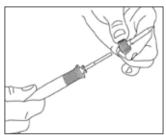
Remove the soldering tip.
