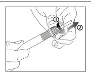
■ Unlock ① and pull off ② the soldering tip.
