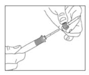
Remove the soldering tip.
