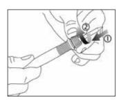
■ Fit the soldering tip ①, overcome the spring force and lock the bayonet mount ②.
