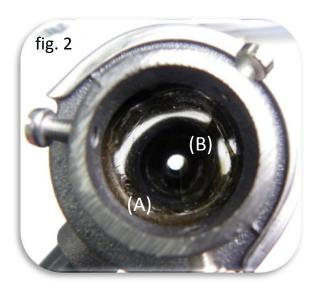
**2.** Check the mica sheets (A) and mica rings (B) for mechanical damage and remove them. (fig. 2)
